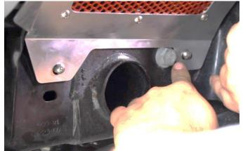
Tighten all visible bolts with a 3mm Allen key.
