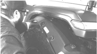
Within the driver side **rear** well, and with a 10mm socket, remove your fuel filler neck bracket bolt. Gently pull the neck loose and push it down below the stud. The passenger side doesn't need to be changed.
