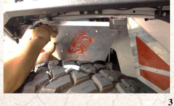
Secure the top with a 16mm bolt, washer, and nut.
