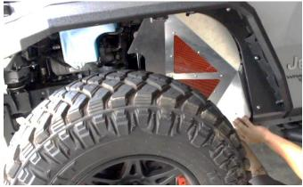
With (2) 16mm bolts and washers, secure the front section to the rear section rivets.
