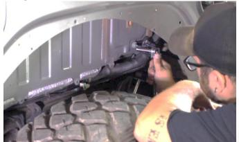
Within the driver and passenger **front** wells, and with a 9/32'' drill bit, expand the two frame holes that are shown below.
