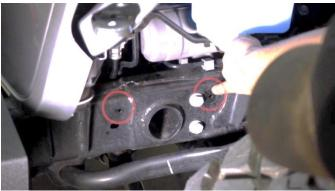
With either an M5 Nutsert Tool **OR** (1) 25mm bolt, M5 hex nut, 10mm washer, and (2) 8mm wrenches, install an included nutsert into each hole.
